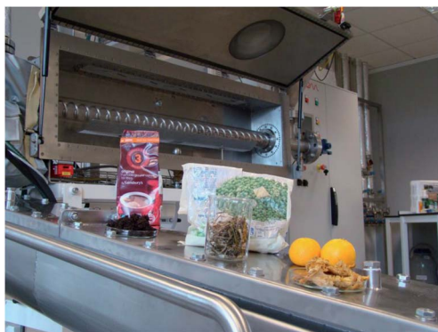
Fig. 5 Examples of waste streams generated by the food manufacturing sector (spent coffee grounds, pea pods and waste citrus peel, from left to right) in front of a 30 kg per hour pilot scale microwave at the Biorenewable Development Center of the University of York.
